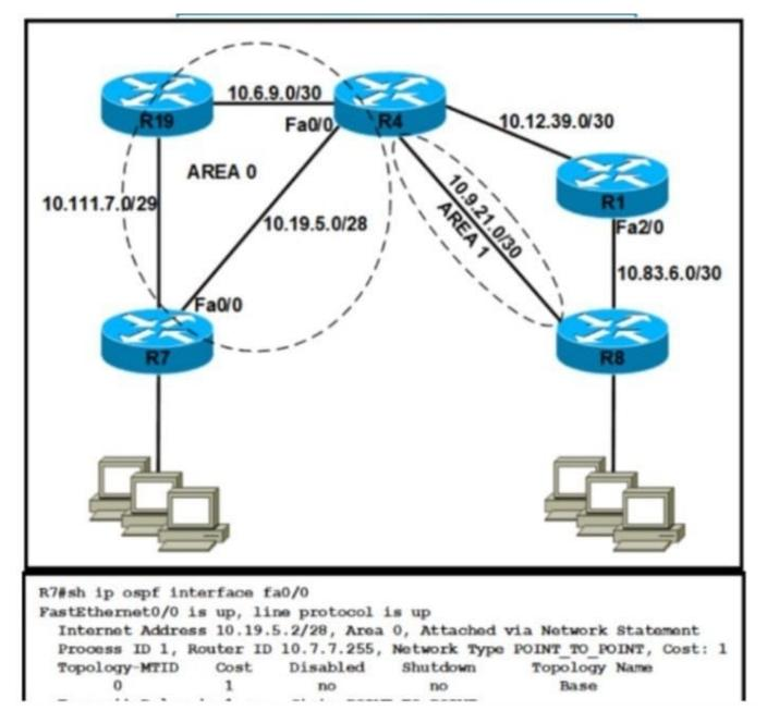
Router R4 is configured correctly with default OSPF values. A network engineer configured R7 for OSPF. R7 must not
